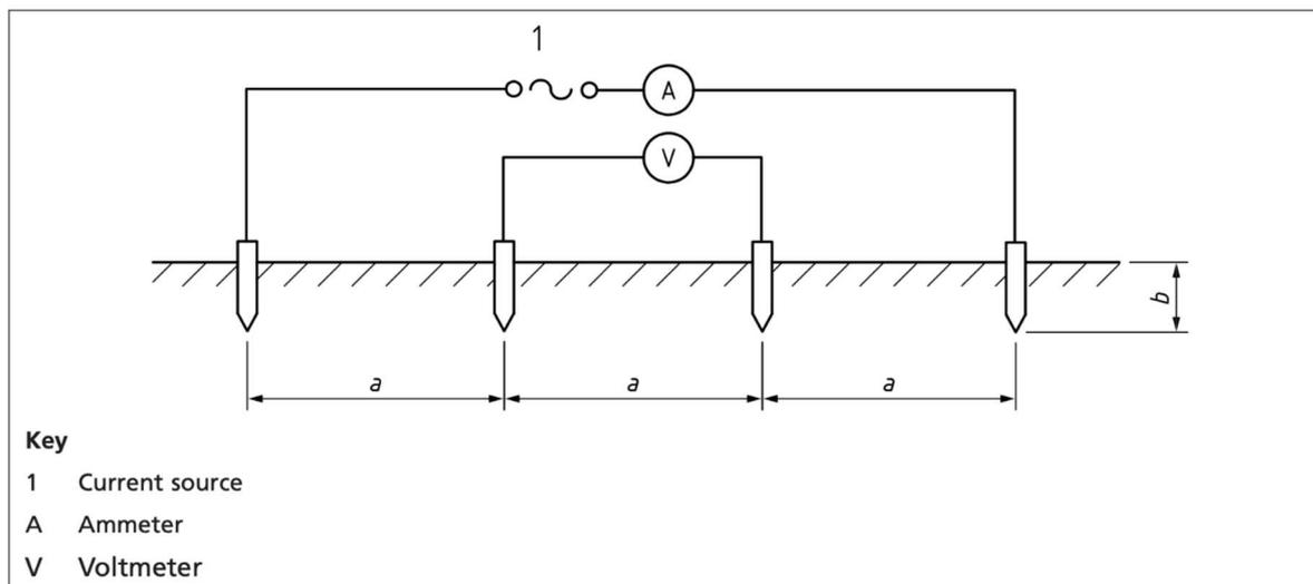
**Figure 1 - Diagram of measurement setup**
