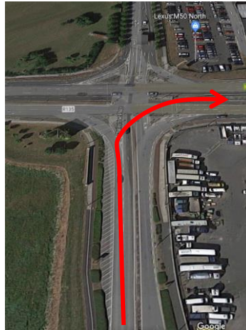
Figure 16 Critical right turn movement at Charlestown Place junction, where an additional lane is recommended.
