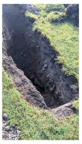
Figure 3-5 LF-TP-2011 Excavation. Visible sandy cap over landfill material
